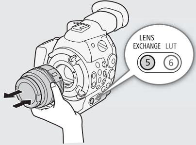
2 Remove the lens attached to the camera and attach the new lens.
